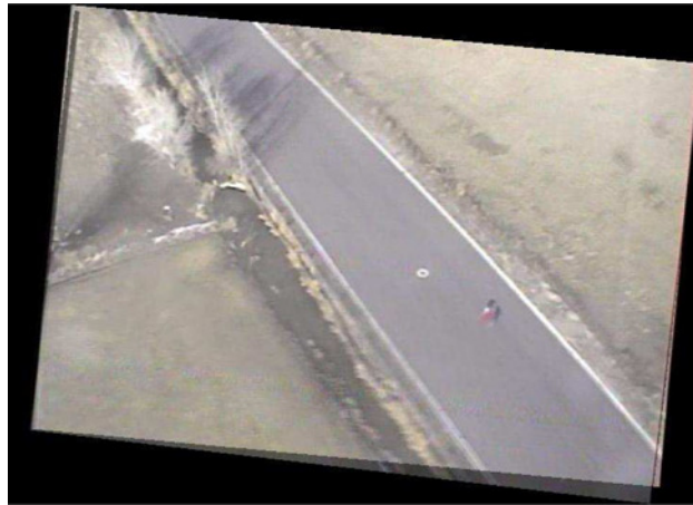
Fig. 17 Two registered video images, one overlaid upon the other, demonstrating proper frame motion estimation.
