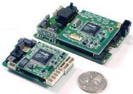
Fig. 4 The Kestrel™ autopilot, versions 1.45 (top) and 2.0, can be reprogrammed to flight test new guidance and control techniques.
